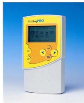
MultiLogPRO can record data from up to 8 sensors simultaneously; it is capable of recording at rates of up to 21,000 samples per second, and of collecting up to 100,000 samples in its internal memory.
